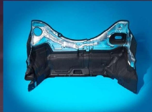
This all-plastic engine-room partition wall provides excellent sound insulation between engine and passenger compartments thanks to the use of long-glass PA 6/6 with barium sulfate. Replacing stamped steel plus a sound-deadening pad, the patented injection-molded plastic partition reduces engine noise 8 dB, lowers part count and assembly time, and offers a 20% weight reduction without increasing costs.
